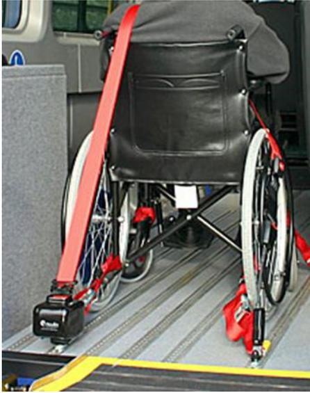
*Wheelchair secured to the vehicle, the passenger is also protected by three-point belt.*
